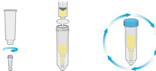
**Figure 1.** Assembling of Anti-EPO gel columns and funnel.
